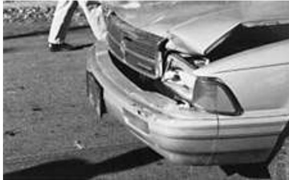
Figure 2 - Damage to Dodge Spirit After Test 9
