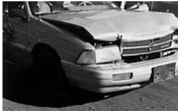
Figure 3 - Cumulative Damage to Dodge Spirit After Tests 9 & 10
