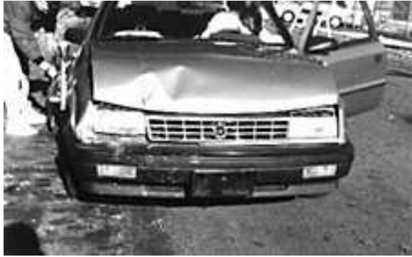
Figure 4 - Cumulative Damage to Plymouth Sundance After Tests 14 & 15
