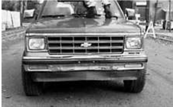
Figure 1 - Cumulative Damage to Chevy S-10 Blazer After Tests 1-5
