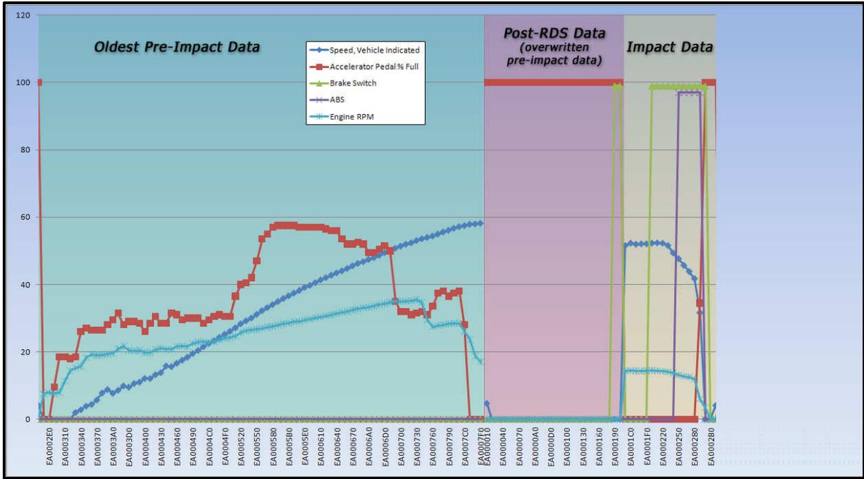
**Figure 8** During the second sort, the post-RDS data and the impact data is placed to the right of the oldest pre-impact data.
