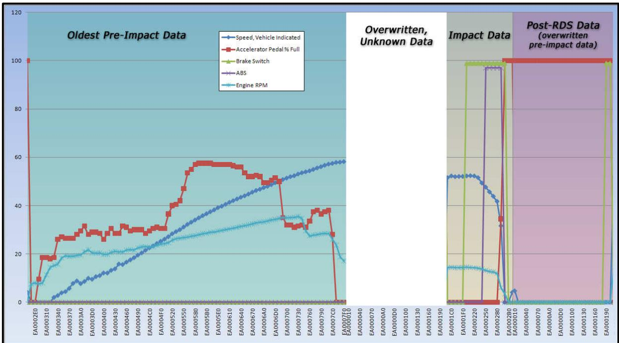
**Figure 9** During the final sort of the data, the post-RDS data is placed at the end of the graph, leaving a blank space between the impact data and the oldest pre-impact data to account for the overwritten pre-impact data.
