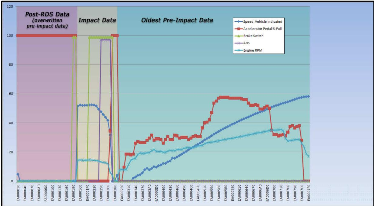
*Figure 7 Data from the example “Locked-Reboot” data file sorted so that it is in its proper memory buffer address order.*
