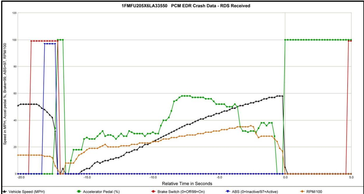
**Figure 5** Example of a “Locked-Reboot” PCM data file. The actual impact can be seen on the left portion of the graph, and has been incorrectly sorted by the CDR software. Manual sorting of this type of file is necessary.
