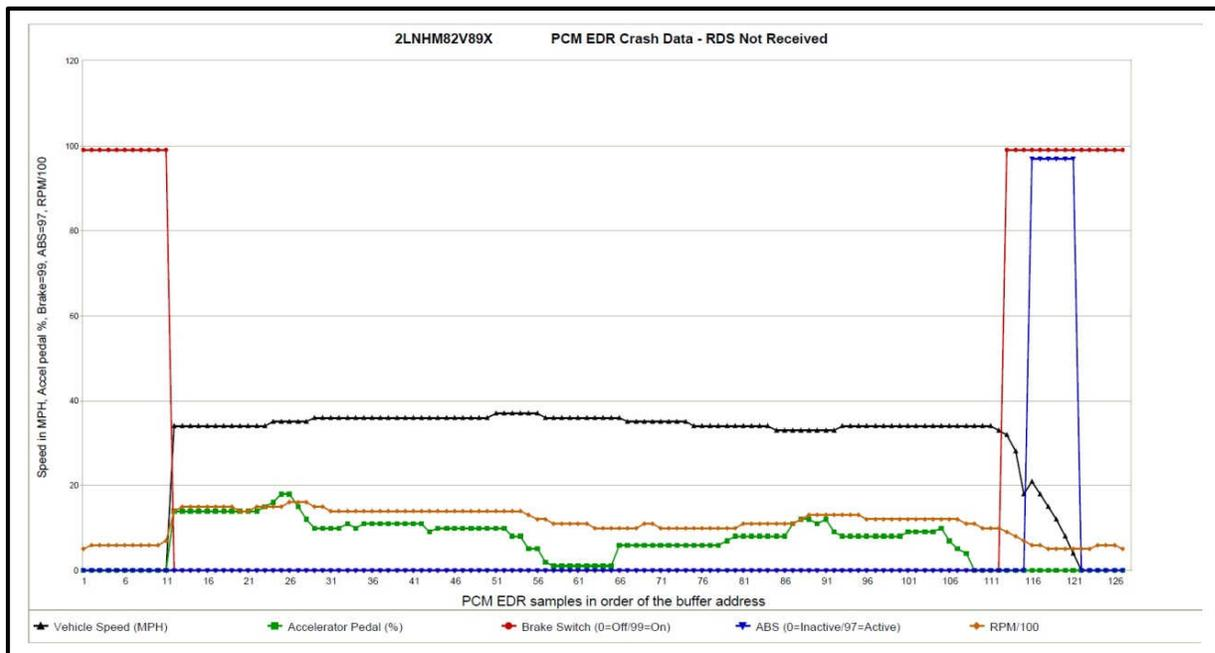
**Figure 2** *An example of an unlocked PCM data file created during a hard braking incident. In order to sort this data into its proper order, the data contained on the left portion of the graph must be placed to the right of the data seen on the right edge of the graph.*
