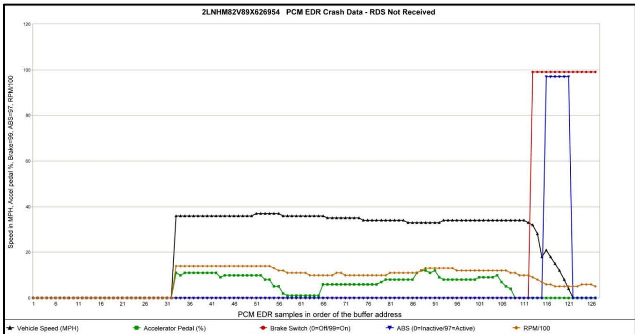
**Figure 3** *An example of an overwrite of data caused by turning on the ignition switch without first attaching the PCM Power Adapter. Note that the overwrite has occurred at the beginning of the memory buffer and continues for several seconds before the ignition was turned off.*
