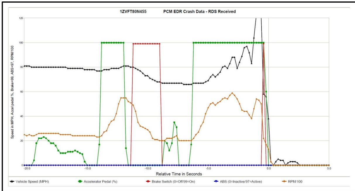
**Figure 1** *An example of a locked PCM data file that has been properly sorted by the CDR software.*
